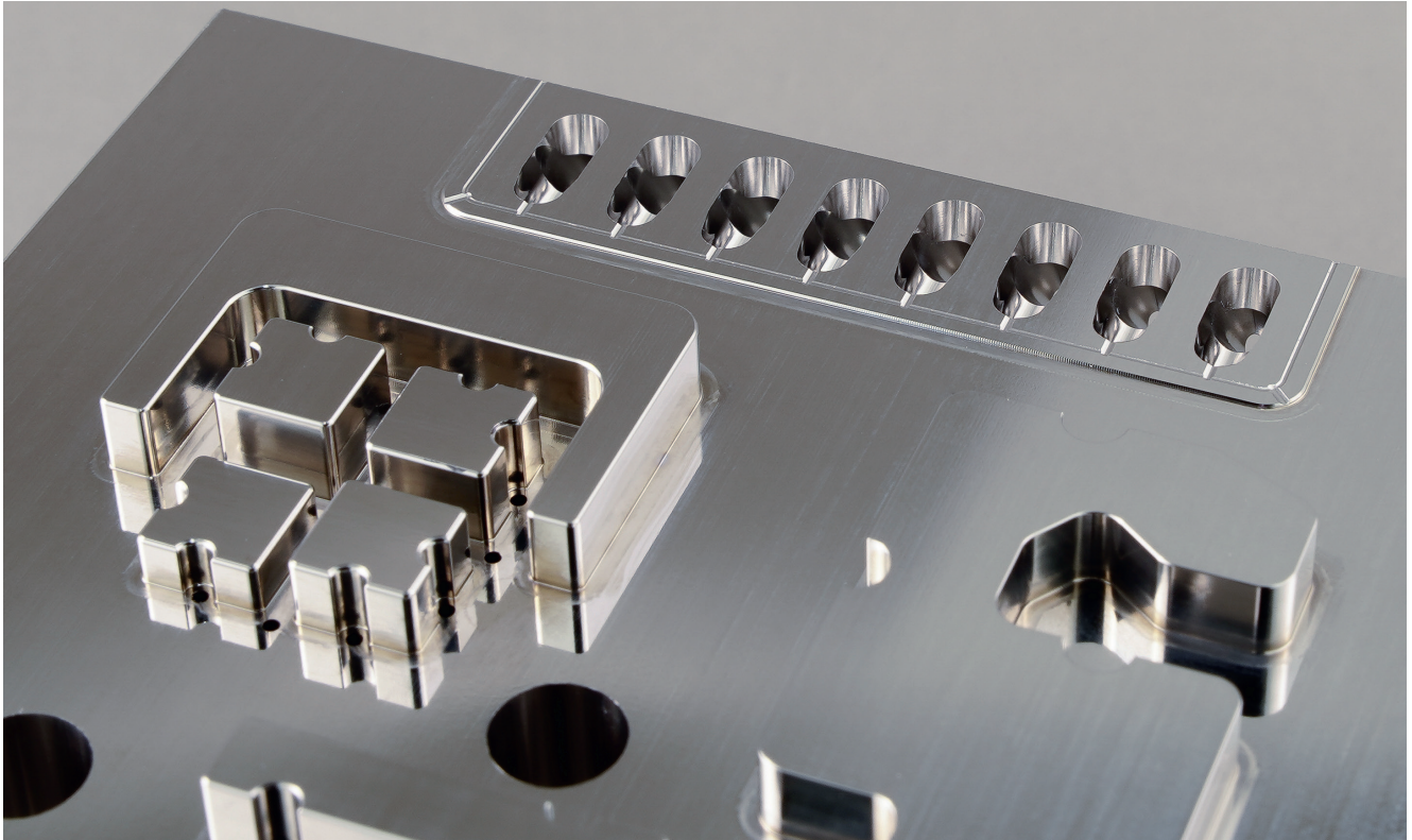
The sprue side of the example tool: All eight sprues were exclusively hard-drilled and milled. For example, the strategy of groove milling was used for the cone, which was also used for milling the three fits with a diameter of 6 mm
