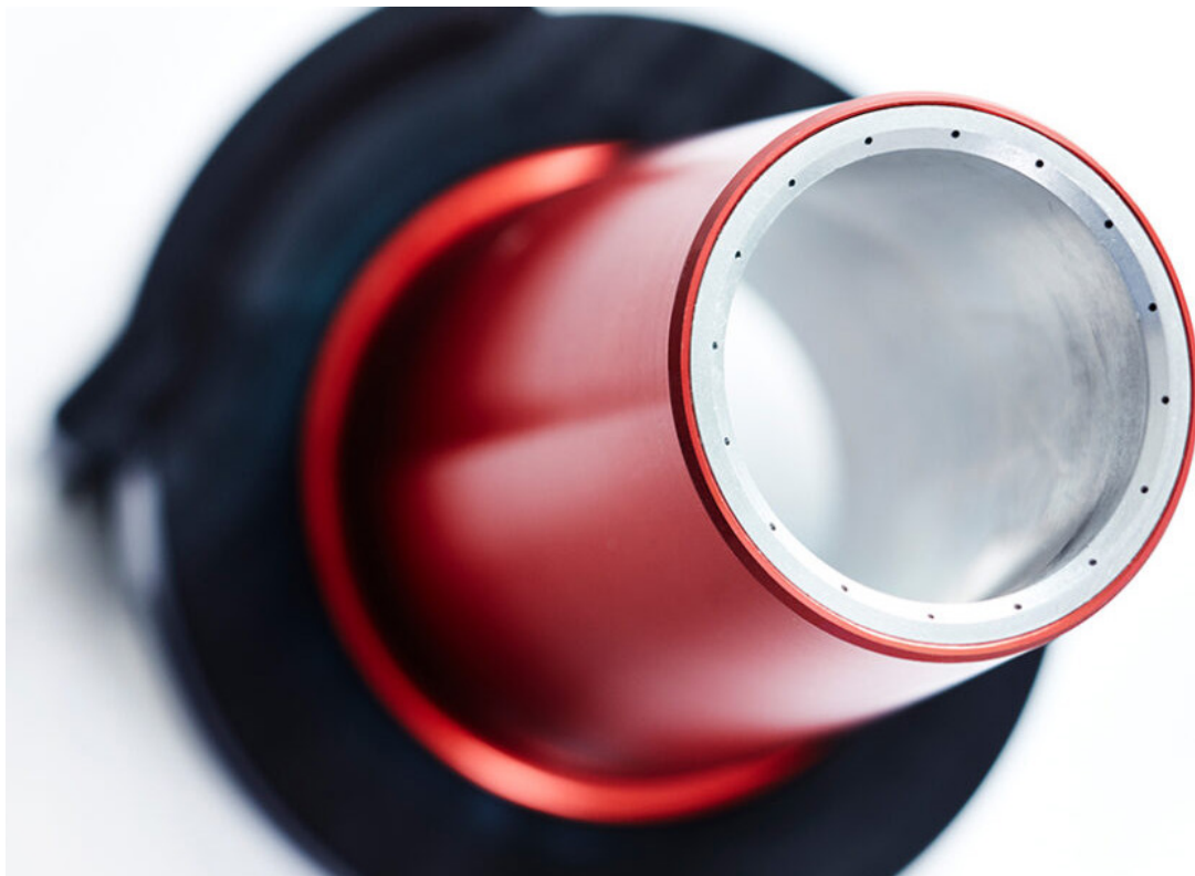
With the medium distributor from MHT (Merz & Haag), a particular air distributor system is used to blow either pure compressed air with a bit of oil compressed air or hydrocarbon medium (MV-2) onto the tool in such a way that it is optimally cooled and the chips are reliably removed.
