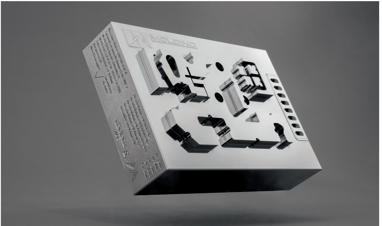
The example mold insert designed by Mark Rotzoll is made of high-strength, ground hot-work tool steel 1.2343 ESR (X37CrMoV5-1 ESR) pre-hardened to 52 HRC.
