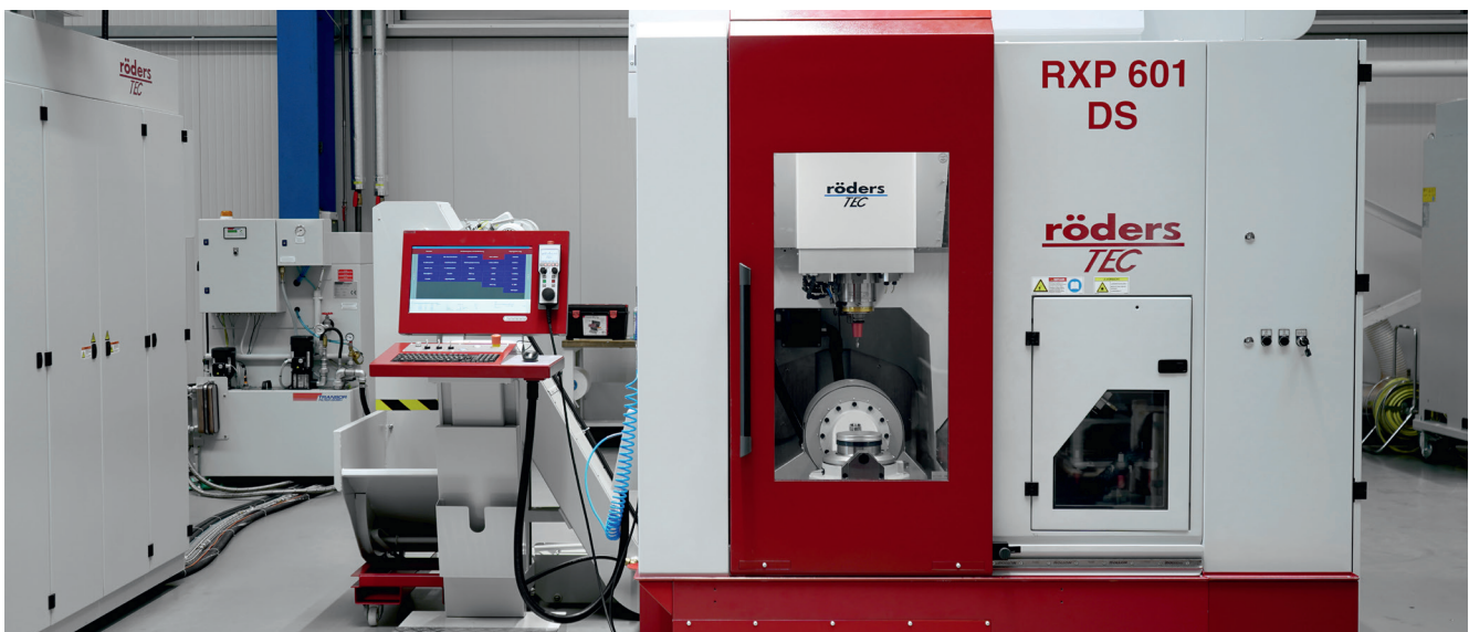
The mold insert was milled in two clampings on the 5-axis Rödgers RXP601 DS, equipped with the medium distributor from MHT.
