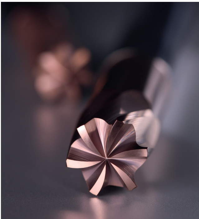
The 4- and 6-flute polygon end mills from the EHHRE series are available in diameters ranging from 0.5 to 12 mm. The applied TH3 coating enables the machining of hardened steels up to 68 HRC.
