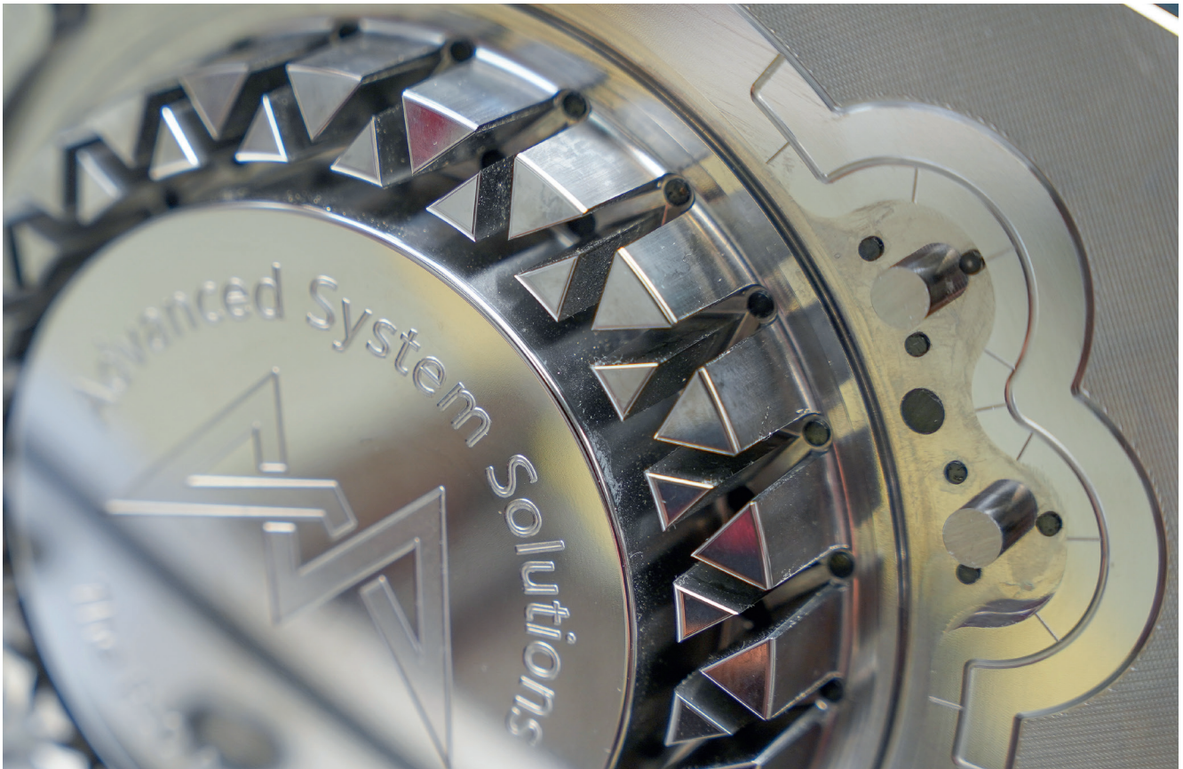
View of the ejector side, showing the ribbing, several of the total 76 ejector holes machined to H7 quality, as well as the mirror-milled cover area. The labeling and logo were engraved using a chamfer cutter from the DN2HC series.
