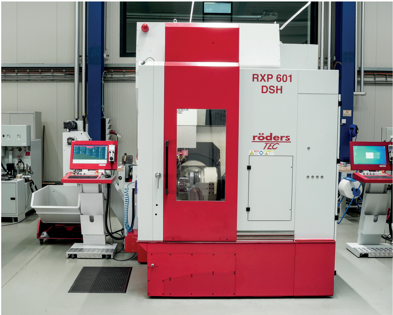
The 5-axis RXP 601 DSH in Röders' application center, on which the majority of the sample assembly was also manufactured in advance.
