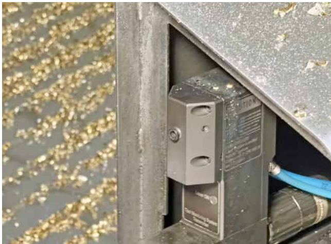
The laser unit for tool measurement is just one of numerous measuring devices that the system uses to monitor itself and optimize the machining processes (Photo: Klaus Vollrath)
