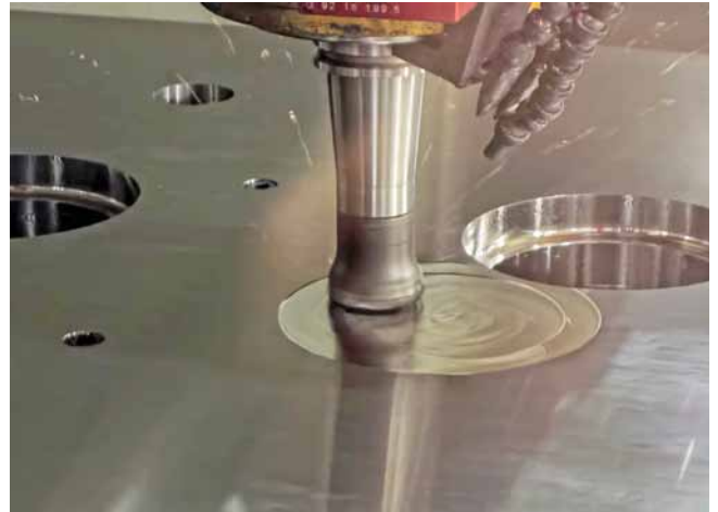
The standard spindle (101 Nm, 22,000 rpm) is milling the test workpiece with a cutter head with a diameter of 52 mm (Photo: Klaus Vollrath)
