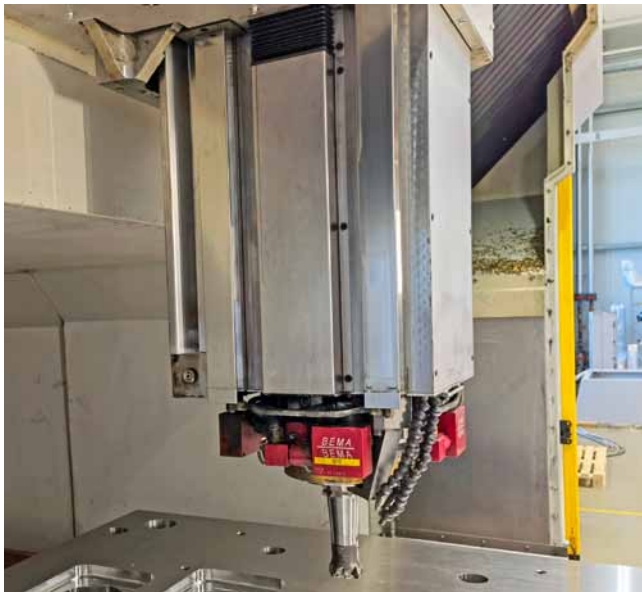
The Quadroguide principle with four guide rails at the four corners gives the Z-axis particularly high rigidity (Photo: Klaus Vollrath)
