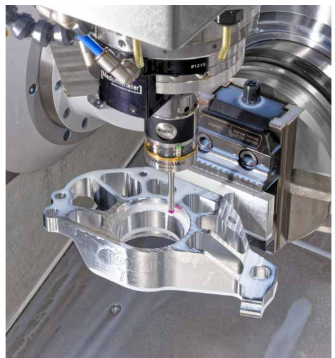
Quality control directly in the machine: Measurement of a workpiece after machining (photo: Roeders GmbH)
