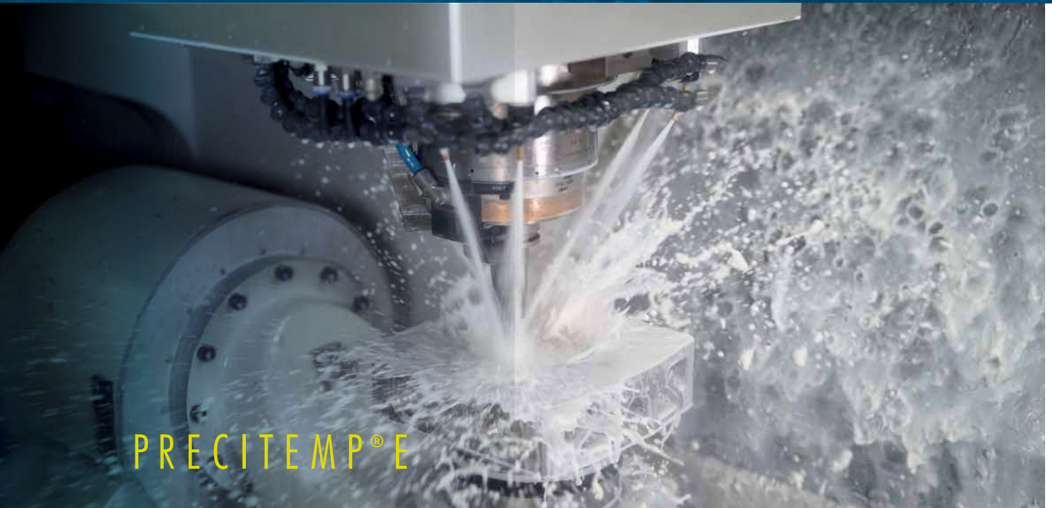
Temperature-stable machining area during machining with emulsion (photo: Roeders GmbH)
