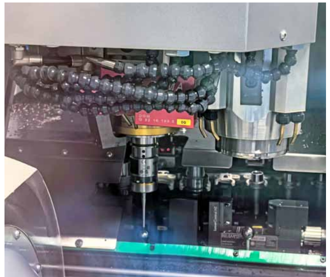
The air-bearing spindle can be seen to the right of the standard HSC spindle (here holding a 3D probe and with open sliding cover). Below it is the second exchanging set with its own probe ball and measuring laser (photo: Klaus Vollrath)
