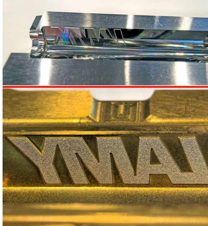
Today, the mold halves are milled from the already hardened blank (above) and briefly polished. After structuring the background by a short EDM machining pass and applying a TiN coating, they are ready for sampling (photo: Klaus Vollrath)
