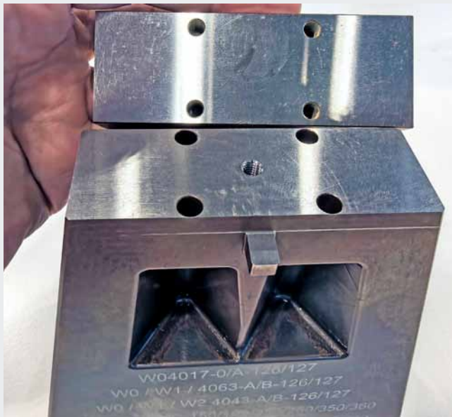
The hardened blanks, which are ground flat only on one side and provided with threaded fixture holes, are fixed to the self-developed workpiece carrier with four screws, thus enabling effective, collision-free five-sided machining (photo: Klaus Vollrath)
