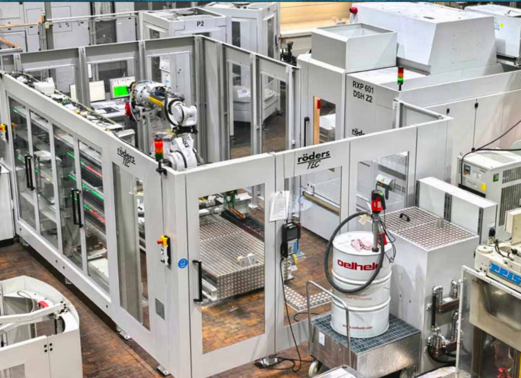
Custom-made: Top right, the RXP 601 DSH Z2 milling center with double spindle; in the middle, the robot; and left, the magazine with workpieces and tools (photo: Klaus Vollrath)
