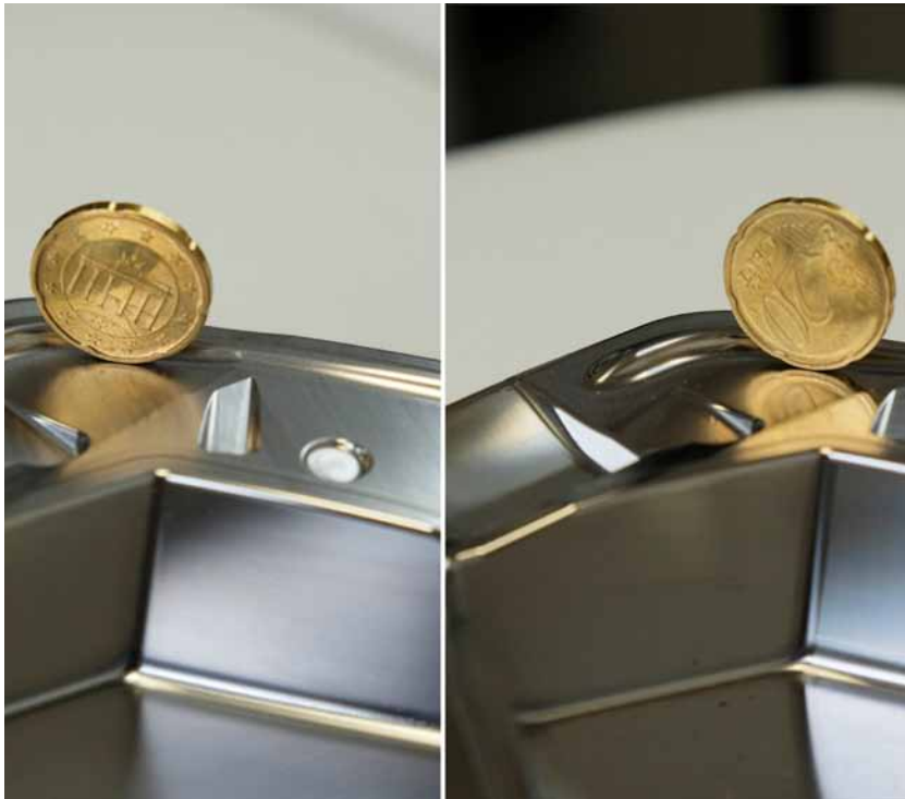
Gloss comparison between a workpiece milled with a conventional approach (left) and a comparative part machined with modern tools and strategies (Photos: MMC Hartmetall)
