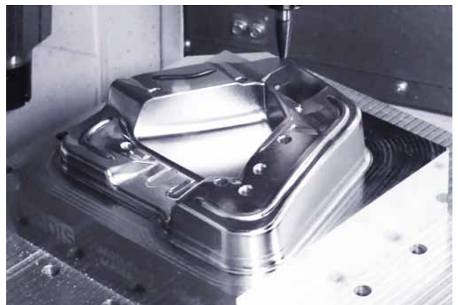
Modern finishing: VHM barrel cutter VQT6URR with 6 cutting edges for highly productive finishing with large infeed (Image: Röders/MMC/Tebis)
