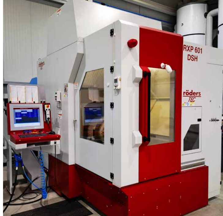
The RXP 601 DSH 5-axis milling centre from Röders used for the machining tests (Photo: Klaus Vollrath)
