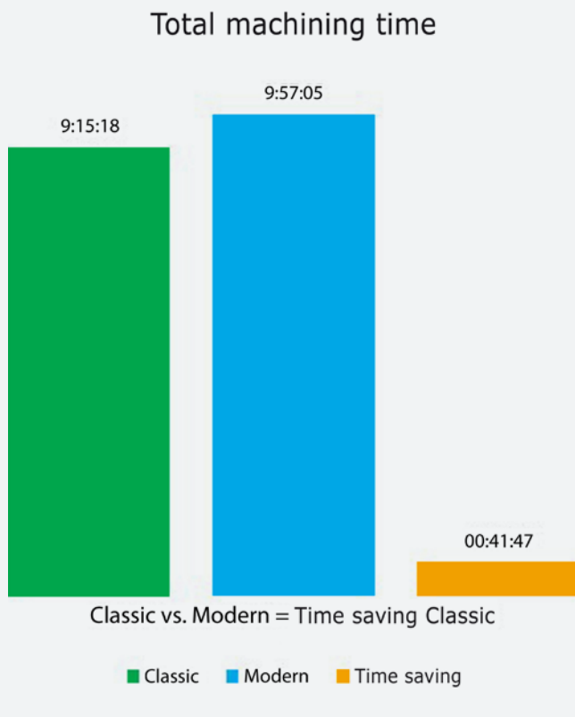
Balancing the machine processing time resulted in a time gain of approx. 42 min for the "classic" approach (Graphic: Tebis)
