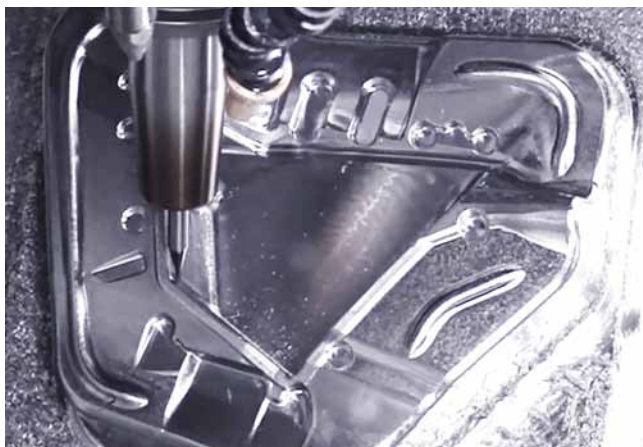
Semi-finishing and classic finishing: solid carbide ball nose end mill MP3XBR with conical neck for semi-finishing and finishing of deep cavities. (Image: Röders/MMC/Tebis)
