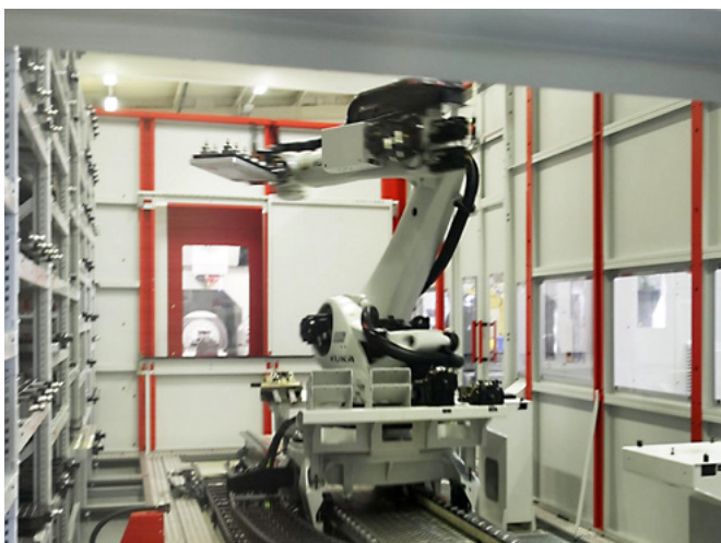
In the milling cell in the Alpla tool shop, a Kuka robot supplies work to the two Hermle C 42 U universal machining centers and a Rödgers RXP 950 DSH high-precision HSC milling machine. - Image: Pergler Media
