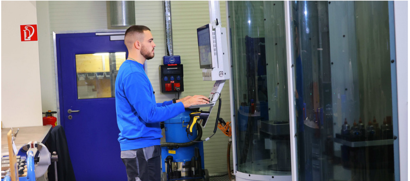
The workers at Alpla set up the electrode blanks and transfer them to the automated milling line. Everything else takes place without operator intervention - the Kuka robot handles the workpieces. And thanks to in-process measuring on the Röders, high process reliability is guaranteed. - Image: Pergler Media
