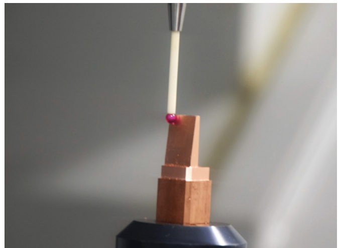
The mold makers generate the measuring points for quality measurement on the Röders RXP 950 DSH directly from Cimatron. In-process measurement guarantees stability and reliability for subsequent processes and ensures the high precision of the sealing surfaces on the injection molds. - Image: Pergler Media
