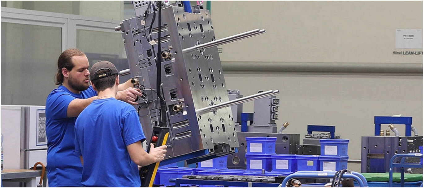
Complex, high-cavity molds for closure caps dominate injection mold making within Alpla's mold shop. High repeatability is important for mold nests - after all, every part should be exactly the same regardless of the cavity in which it is injected. - Image: Pergler Media
