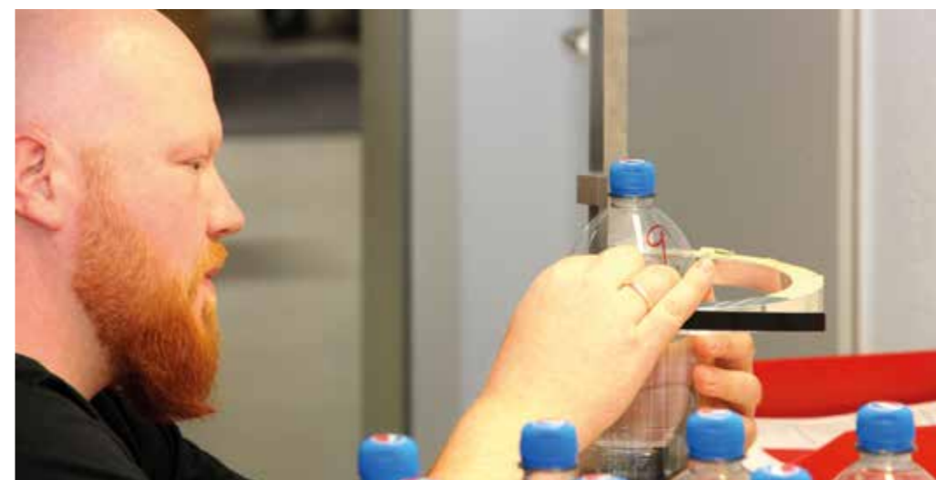
Fig 3: Dimension check after 24 hours in 38°C chamber
